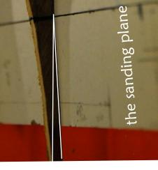
The plug is sanded until the glue lines show in the right Place. This is checked by the plan to the right scale drawn On tracing paper to compare them.
