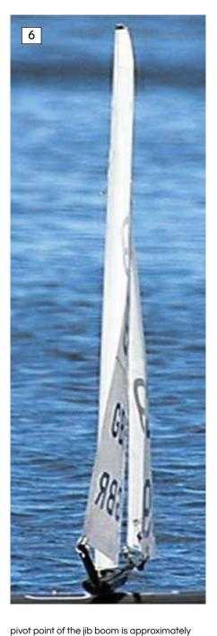
camber so that the angle of the back of the jib doesn't impinge onto the mainsail, as this will encourage back winding of that sail, which is not a good idea. The wind needs to funnel through the gap or slot between the two sails without undue restriction.
